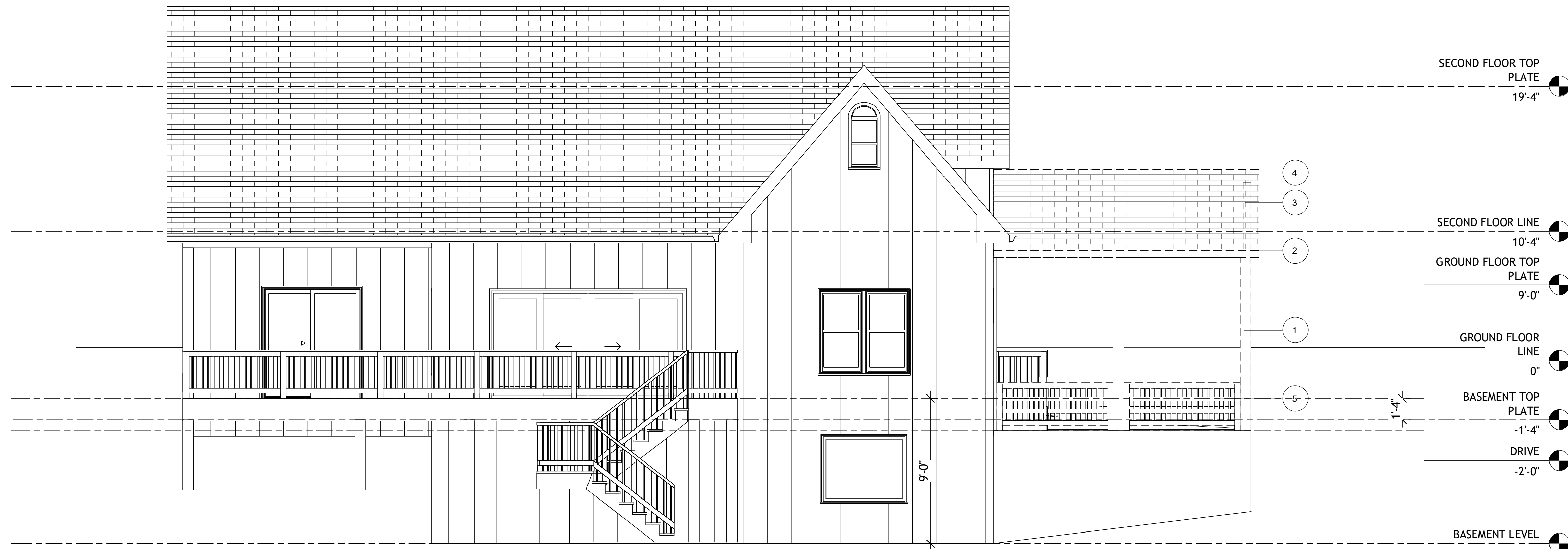
1 REAR ELEVATION DEMO A2-01 1/4" = 1'-0"
