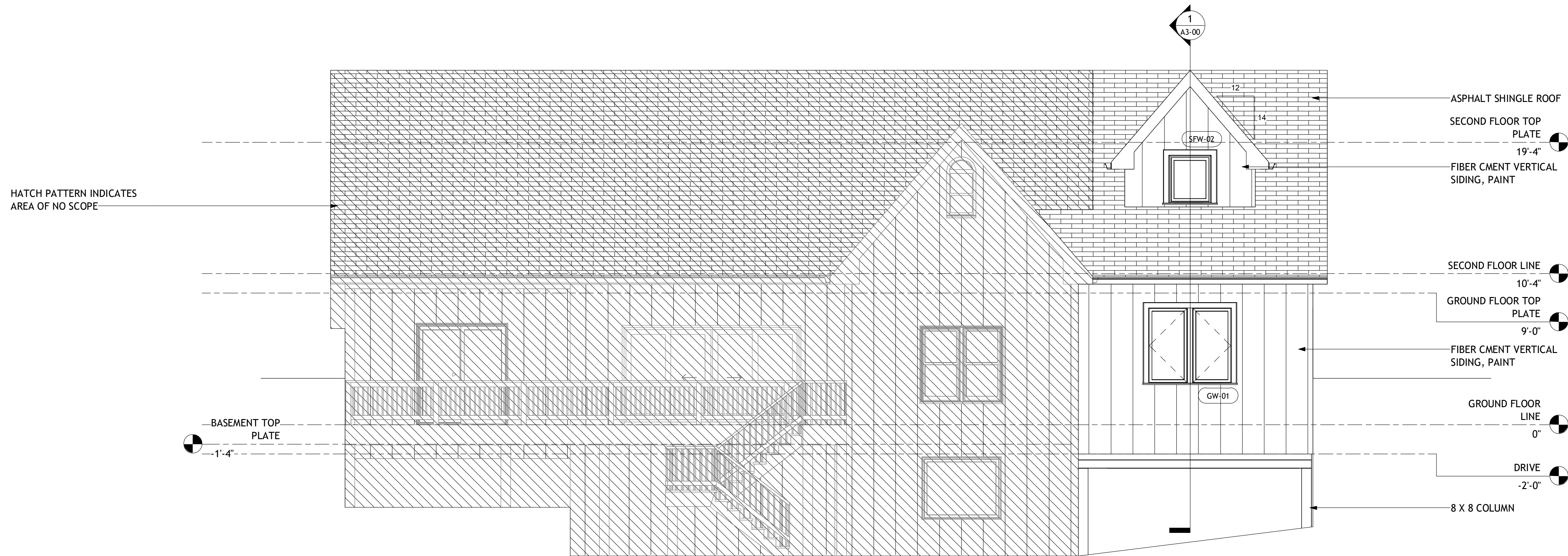
1 REAR ELEVATION PROPOSED A2-03 1/4" = 1'-0"
